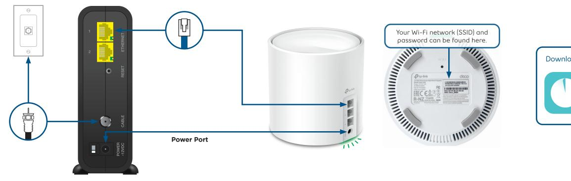
(!) If the light is **red**, reboot the modem and Wi-Fi pod by unplugging the power adaptors.
